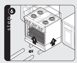
Lift unit and prop on wood blocks.
